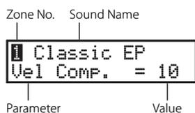
Zone parameters can be edited individually for each zone. There are two parameter groups, Internal parameter group and External parameter group. If a zone is set to Int, only Internal parameters are available for editing. If a zone is set to Ext, only External parameters are available for editing. If a zone is set to Both, both Internal and External parameters are available for editing.
