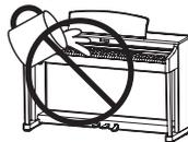
Entry of water, needles or hair pins may result in breakdown or short-circuit. The product shall not be exposed to dripping or splashing. No objects filled with liquids, such as vases, shall be placed on the product.
