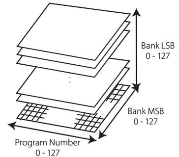
This is a 3D image of the expanded program change system with the MSB and LSB. To use these efficiently and correctly, refer to the operation manual of any external MIDI sound modules that are connected to the MP6.
